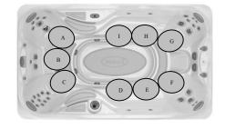
LISTED DIMENSIONS REPRESENT DISTANCE FROM THE TOP OF ACRYLIC TO LOWEST POINT IN THE SEAT. TOLERANCE  $\pm 1/16$ " (0.158CM)
